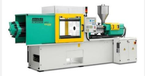
Medbio is pleased to announce the delivery of our 22nd press on January 18th. Our latest addition is a new Arburg 470C-165 ton hydraulic molding press with a 5oz shot size. This new machine will add both redundancy and additional capacity to our molding capabilities, and will be used for some of our higher volume work.
